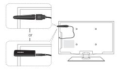
To reconnect the Samsung Wireless LAN Adapter using the extension cable, follow these steps:
